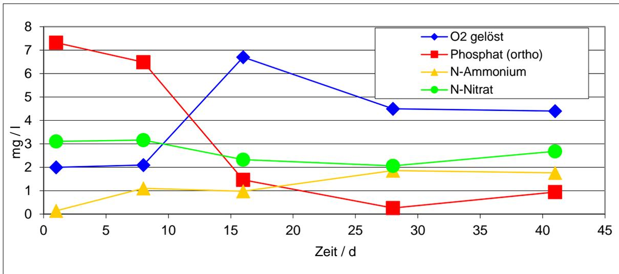
The dissolved oxygen content stabilizes after 3 - 4 weeks at a level of 4 mg/l, which corresponds approximately to twice of the initial value of about 2 mg/l. The content of phosphate decreases from 6 mg/l in a first phase to values below 2 mg/l, and then stabilises at 2 mg/l. The nitrate concentration decreases slightly, and accordingly to the ammonium nitrogen content increases slightly (compare with Figure 2).
